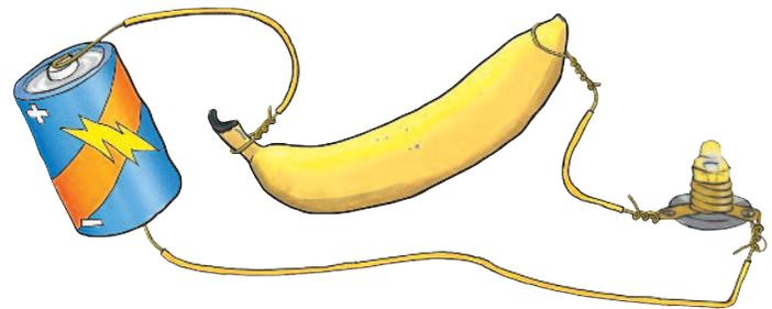
1. Get a 1.2-volt light bulb, a matching light bulb base, a D-cell battery, a banana, and three pieces of copper wire with the insulation stripped off the ends. Ask an adult to help you strip the insulation.
